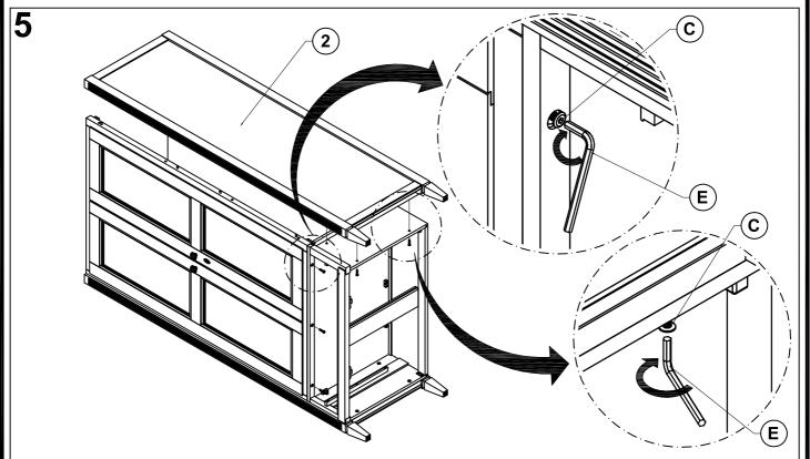
Use 4x bolts 30mm to fix the drawer box to RH side panel and 3x bolts 30mm to fix the drawer box to door frame set - as shown
